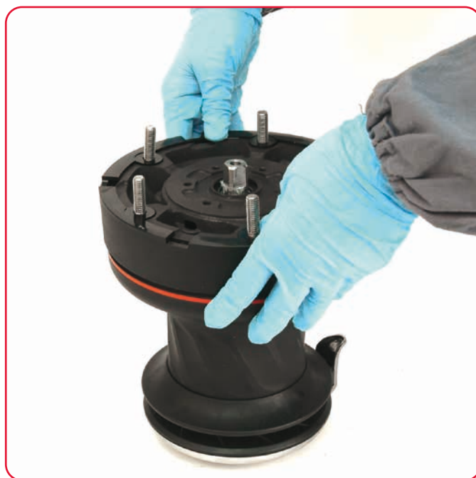
5. Press down the skirt to position it correctly
