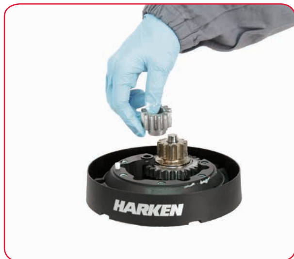
8. Remove the gear
