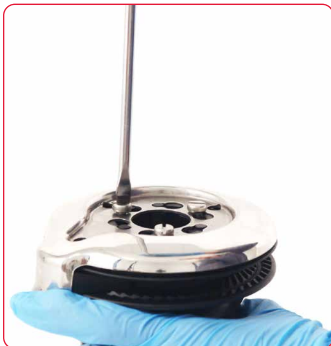
3. Unscrew the three screws (4Nm/35 in-lb).
