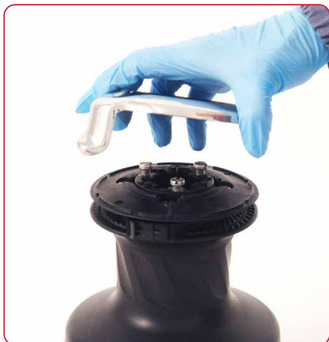
4. Remove the self-tailing arm by rotating and lifting it.
