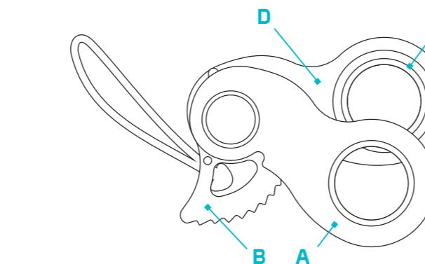
**EN:** (A) Mobile bracket in aluminium alloy, (B) Clamping cam in steel, (C) Drum in steel, (D) Main plate in aluminium alloy.
